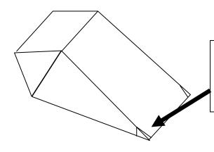
Here is where one the axels for the wheels is placed when building your car after you have cut off the edge, your other axel is attached to the motor at the other end of the car
